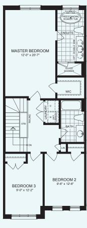
SECOND FLOOR PLAN ELEVATION A1
